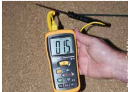
Monitor moisture and temperature using a digital probe
